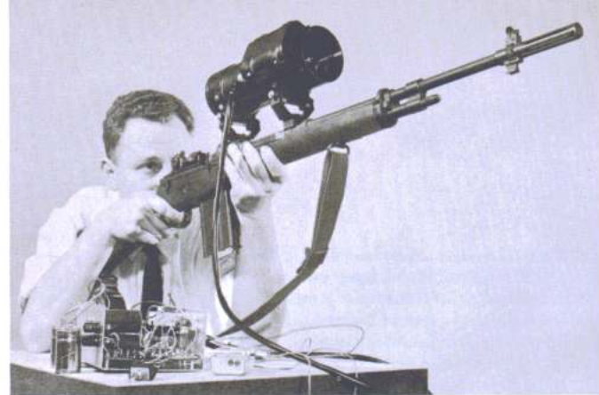
New training device for infantrymen under development at Bulova is this infrared-rifle that "shoots" other soldiers with beams of infrared — hits are registered by beams instead of bullets. Power source and detection equipment will be "packaged" in a canteen-size container that soldiers can carry on hip.
