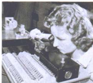
Tiny coils are wound with spiderweb-like wire drawn by Bulova because no outside source could meet the rigid requirements of the Accutron electronic circuitry. Each coil contains 8,000 turns of wire which is one-fifth the thickness of a single human hair.
