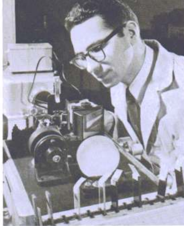
Sample filters needed for military optical systems are being checked by Bulova physicist who is calibrating monochrometer unit of new spectrophotometer.
