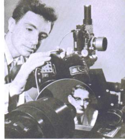
Scanning radiometer simulator is typical of Bulova-developed equipment needed for analysis of advanced fire control system design.
