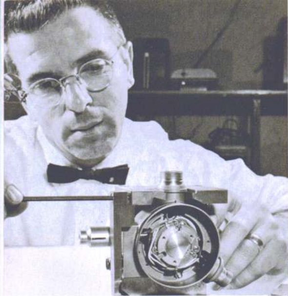
Missile engine igniters for Minuteman are checked after individual environmental testing to assure safety before launch, and to insure reliable ignition at launch and during flight. The Bulova Laboratories is developing other similar electro-mechanical devices for solid-propellant engines.
