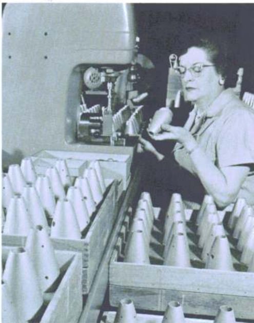
■ Mortar fuzes by the hundreds are being manufactured at the Jackson Heights Plant utilizing machine tools and techniques developed by the precision watch industry.
