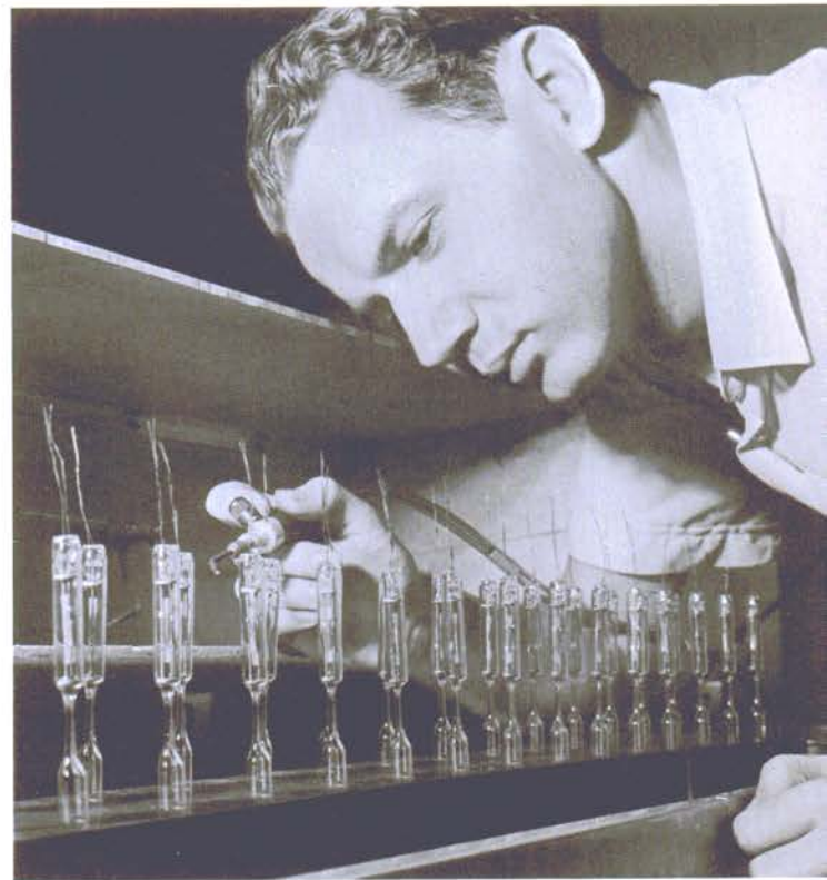
For Guidance Systems —Bench operator Edgar Cadavid, a technician in the Electronics Division's Crystal Department, seals precision quartz crystal oscillators in evacuated glass tubes. These high frequency crystal oscillators are used in helicopter and other guidance systems.
