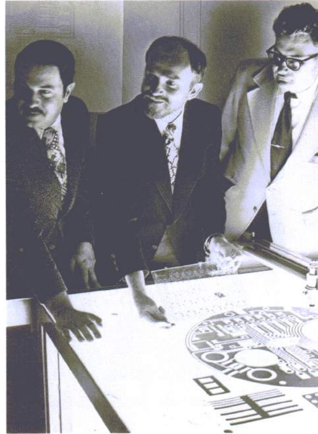
CIRCUITS— Senior technician (above) examines multiple photo masks for printed circuit boards used in solid-state watches. Photo mask is reproduced photographically from giant ruby-lith master (right) inspected by (l. to r.) Robert Sagarino, manager, Product Engineering Department, Dr. Dale R. Koehler, manager of the Advanced Research Laboratory, and William Salmre, senior staff engineer.
