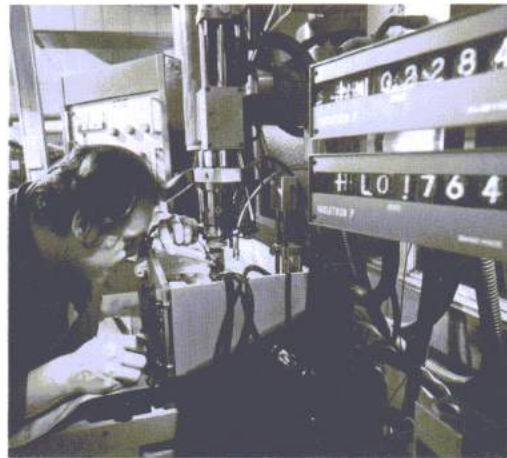
DIE CUTTING—To achieve electronic watch-part tolerances ranging to one ten-thousandth of an inch, engineer uses digital readout electrical discharge machine.
