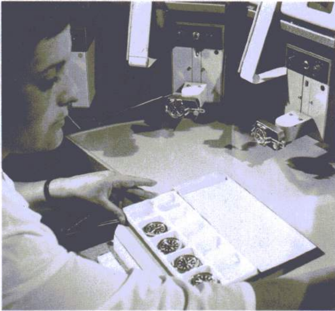
ALL POSITIONS—Bank of electronic machines uses continuous tape to record accuracy of new watches, simulating performance in actual use.
