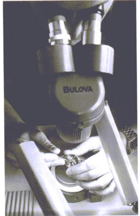
FOR MINI—Electronic equipment measures frequency of tiny mini Accutron tuning fork, permitting technician to assure exact frequency performance.
