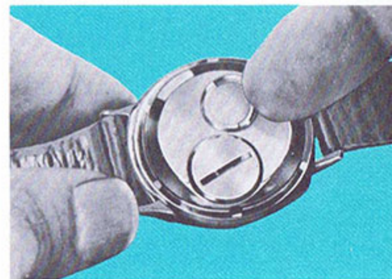
Fig. 2 Lifting the Setting Handle
